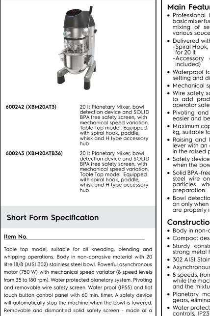
bisphenol-A free (BPA) copolyester. Bowl detction device allows the mixer to switch on only when the bowl and the safety screen are properly installed and positioned together. Adjustable feet for stability. Equipped with accessory drive hub type H (accessories are not included).
